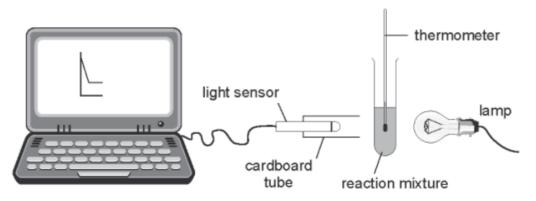
5 cm<sup>3</sup> of dilute hydrochloric acid was added to 10 cm<sup>3</sup> of sodium thiosulfate solution at 60  $^{\circ}$ C and the light intensity was measured over time. The results are shown on the grid below.
