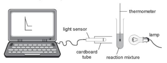
$5 \text{ cm}^3$  of dilute hydrochloric acid was added to  $10 \text{ cm}^3$  of sodium thiosulfate solution at  $60 \text{ }^\circ\text{C}$  and the light intensity was measured over time. The results are shown on the grid below.
