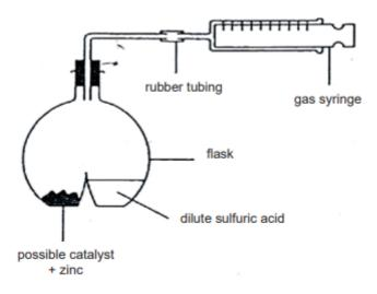
To start the reaction, the flask was shaken. The time taken to collect 50  $\rm cm^3$  of hydrogen was recorded. Other observations are shown in the table.
